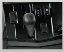
Shift Control Lever with integrated park position makes this our easiest, most accurate shifting Gator UV yet. Electronic 4WD and differential lock engagement lets you gain traction the instant you need it with the flip of a switch.
