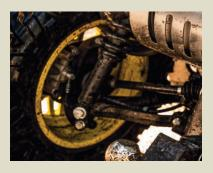
High-strength cast-iron knuckle and upper A-arm support the high stresses of the shocks, constant-velocity (CV) shaft, and wheels in rocky terrain.
