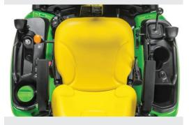
THE CONTROLS are located at hand next to the fenders and color-coded for easy identification
